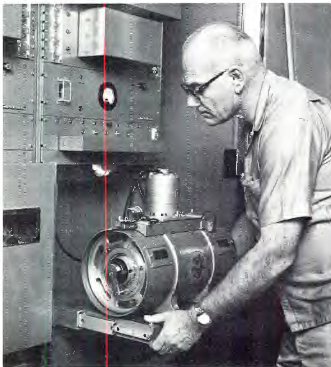
Dirks prepares to check one of the automatic voice announcers used to identify the station.
